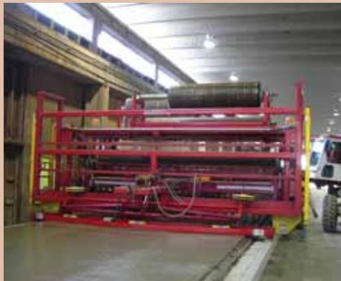
AltusGroup precasters use a patent-pending C-GRID Embedment Machine that introduces carbon fiber grid into the flanges at the optimum depth for crack control and smoothes the concrete in preparation for final finishing. The automated process streamlines double tee manufacturing and ensures optimal placement of C-GRID in the flange.
