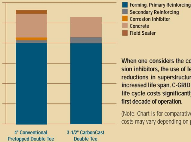
When one considers the cost of steel, and corrosion inhibitors, the use of less concrete, potential reductions in superstructure and site costs, and increased life span, C-GRID reinforcing can lower life cycle costs significantly—especially after the first decade of operation.
