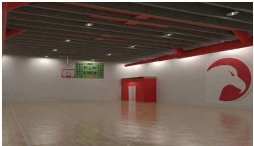
This BIM drawing shows the FEMA safe room designed for the Nixa School district in Nixa, Mo. Originally planned as a 10,000-square-foot building constructed of block and bar joists, Toth and Associates redesigned it as a total-precast concrete structure to convert it into a FEMA safe room eligible for federal funding. Only 4,000 square feet qualified for funding, but that savings, combined with cost efficiencies of the precast concrete design, made the new plan cheaper while also providing the safe-room benefits. BIM drawing: Toth and Associates
