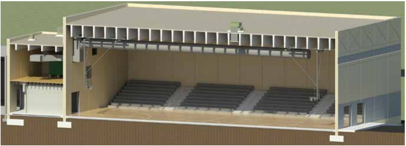
This cutaway BIM drawing shows a gymnasium with a total-precast concrete structural system designed as a FEMA safe room for the Marquand Zion School District in Marquand, Mo. The 1,400-square-foot, two-story addition on the side of the 8,000-square foot gym qualifies as part of the safe room but contains restrooms below and mechanical systems above that feed into the gym. Photo: Toth and Associates
