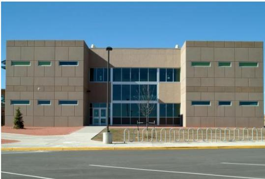
The architect designed an interesting reveal pattern to create an aesthetically pleasing facade. Light sandblasting minimized the potential color inconsistencies of an unfinished colored concrete and produced the appearance of a natural stone texture. Treated with an acid wash, horizontal bands contrast with the sandblast finish to further enhance the exterior.
