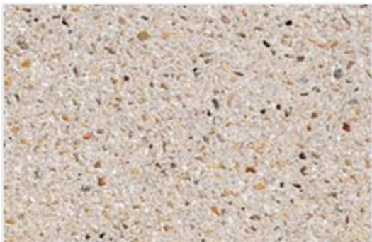
An architectural concrete mix of local aggregates, sands, and fines was given an acid etch finish to ensure that the color and texture of the new addition would match those of the original structure. Continuing the reveal pattern also played a role in minimizing the scale of the six-and-a-half-level parking facility.
