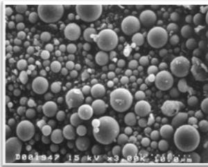
Figure 3 - Fly Ash Particles at 2,000x Magnification
