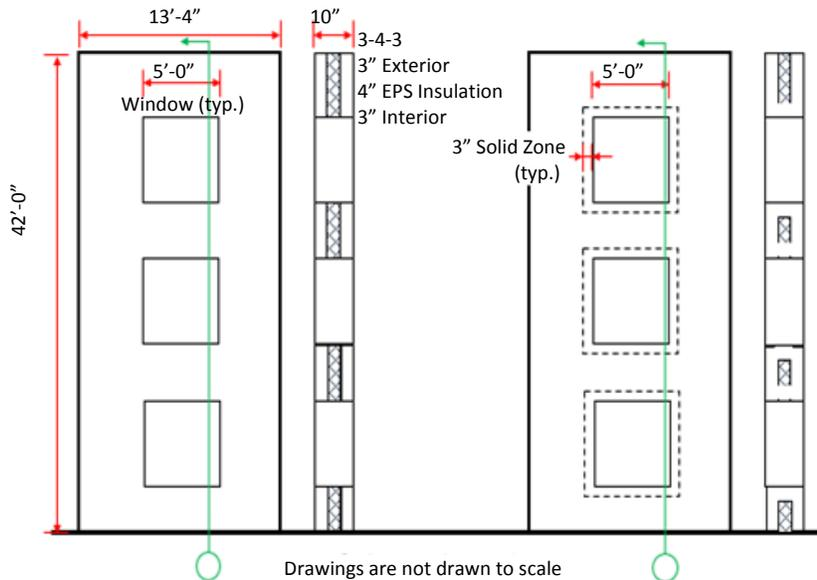
Figure 3: Wall Panel Elevation and Section View through Window
