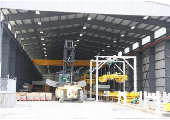
A recent 32,000 square feet of additional precast production area was added to the EnCon Washington facility to house the carousel production system required to produce the tunnel segments. The carousel production system contains nine manufacturing stations, a curing chamber, evacuation line, automated concrete delivery and placement. The batch plant delivers concrete to a casting cabin with a flying bucket and 100% of the waste water is reclaimed and processed through a water treatment plant.
