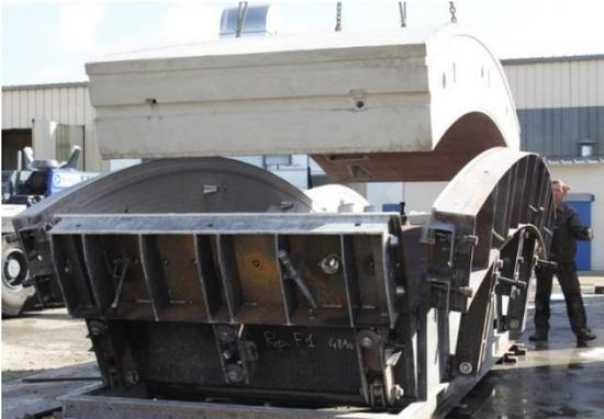
Target production requirements for the tunnel pieces are 33 segments per shift. There are two daily shifts, running 8-9 hours each, allowing for up to 66 segments per day.
